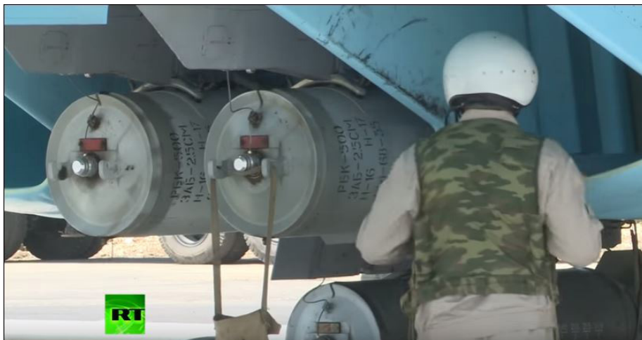
Footage showing what Human Rights Watch arms experts have identified as RBK-500 ZAB-2.5SM incendiary bombs mounted on a Russian attack aircraft at a Russian air base in Syria, 18 June 2016. © 2016 Russia Today/YouTube
